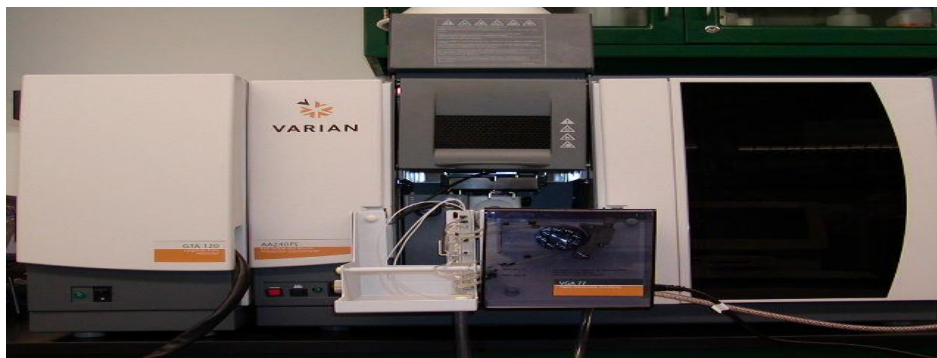
Figure 2: VARIAN 240FS Atomic Absorption Instrument (VGA 77 attached)
